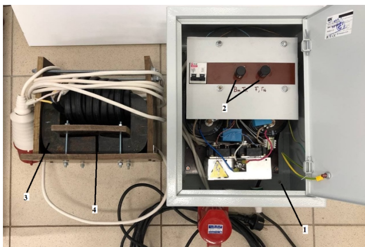
Figure 2 – Pulsed magnetic installation. 1 – control station; 2 – adjustment of magnetic induction and frequency; 3 – electromagnet; 4 – magnetic gap
